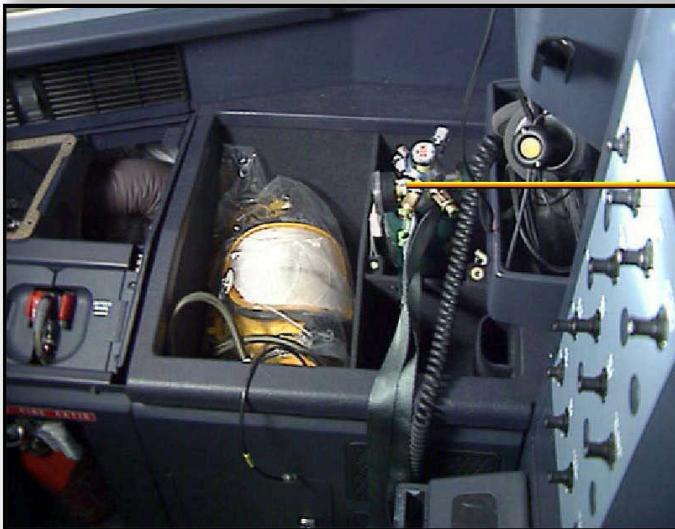
Figure 23 Quick Donning Mask with Portable Oxy. Cylinder
